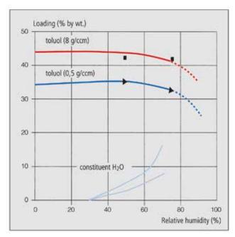
Fig. 6 Influence of relative humidity on adsorption capacity
