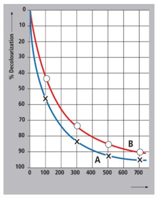
Fig. 10 Decolourization curves of two different activated carbon - Types A and B
