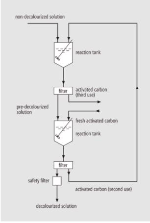
Fig. 11 Two-stage applications of powdered activated carbon
